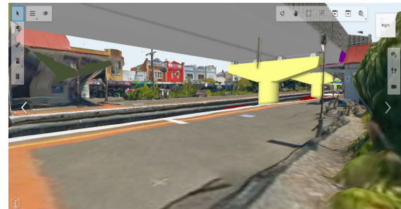
Figure 09. Checking Vertical Clearance using a Digital Twin
