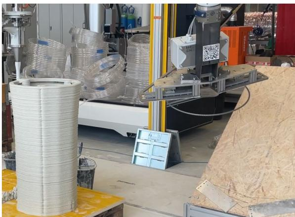
Figure 5. Robotic placement of transverse reinforcement.
