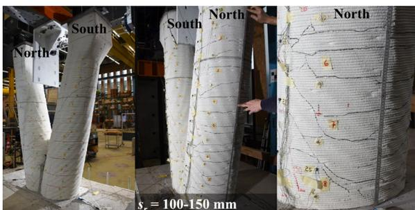
Figure 12. Crack pattern in Specimen *S*: after *Load Case 1* (red) and after *Load Case 3* (black).
