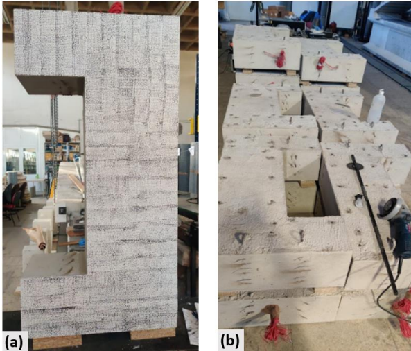
Figure 12. a) Prepared DIC surface b) Prepared top concreting face with steel pins for extensometer gauges.
