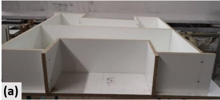
Figure 10. a) Formwork for 1 specimen b) Finished formwork for several specimens.
