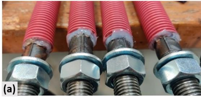
Figure 9. a) PVC tube glued to rebar b) Duct tape at the ends to ensure waterproofing.
