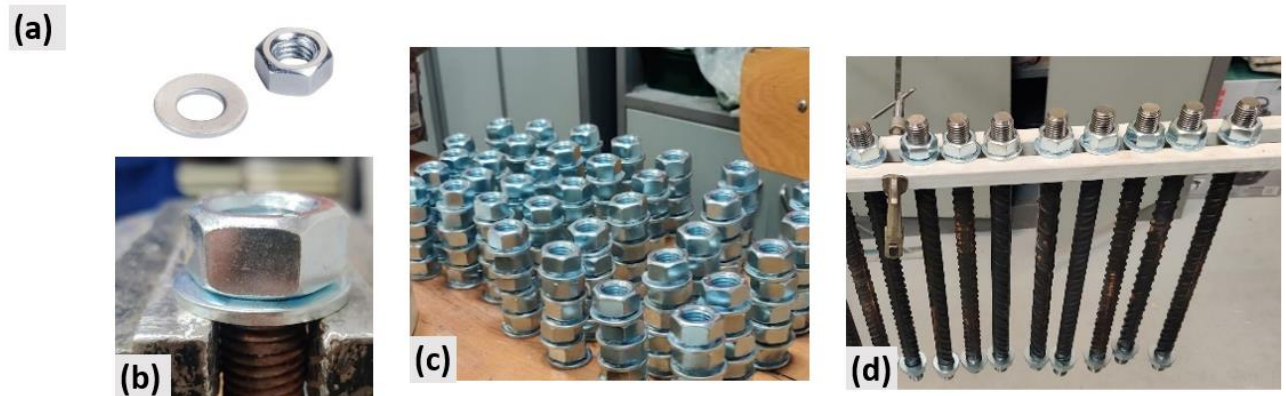
Figure 7. a) M20 Nut and Washer b) Nut and washer placement for hot glue connection c) Glued Nut and bolt d) Positioning of nut and washer on rebar.
