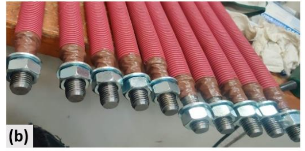
Figure 9. a) PVC tube glued to rebar b) Duct tape at the ends to ensure waterproofing.
