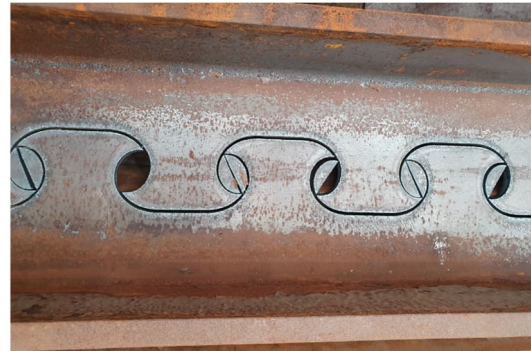
Figure 2. Steel dowels after cutting
