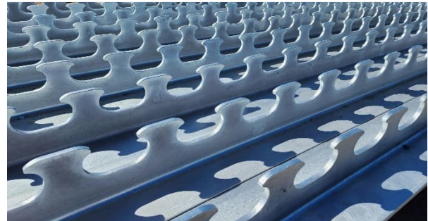
Figure 13. Steel beams with dowels after galvanising
