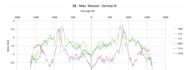
Figure 12. South bound box. Service III (tension) check.
