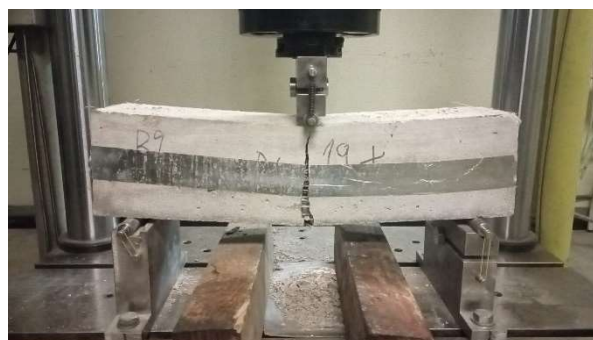
Figure 6. Typical observed failure a) corroded beam, b) uncorroded beam
