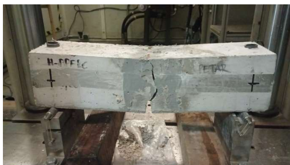
Figure 6. Typical observed failure a) corroded beam, b) uncorroded beam
