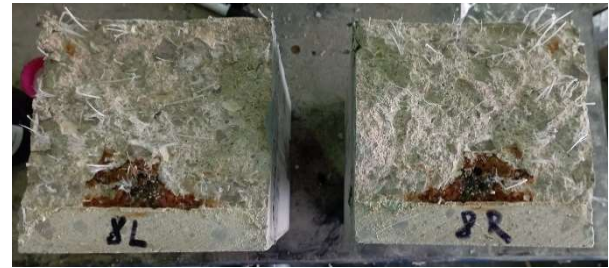
Figure 8. Typical cross section of a corroded beam (pre-cracked and exposed)
