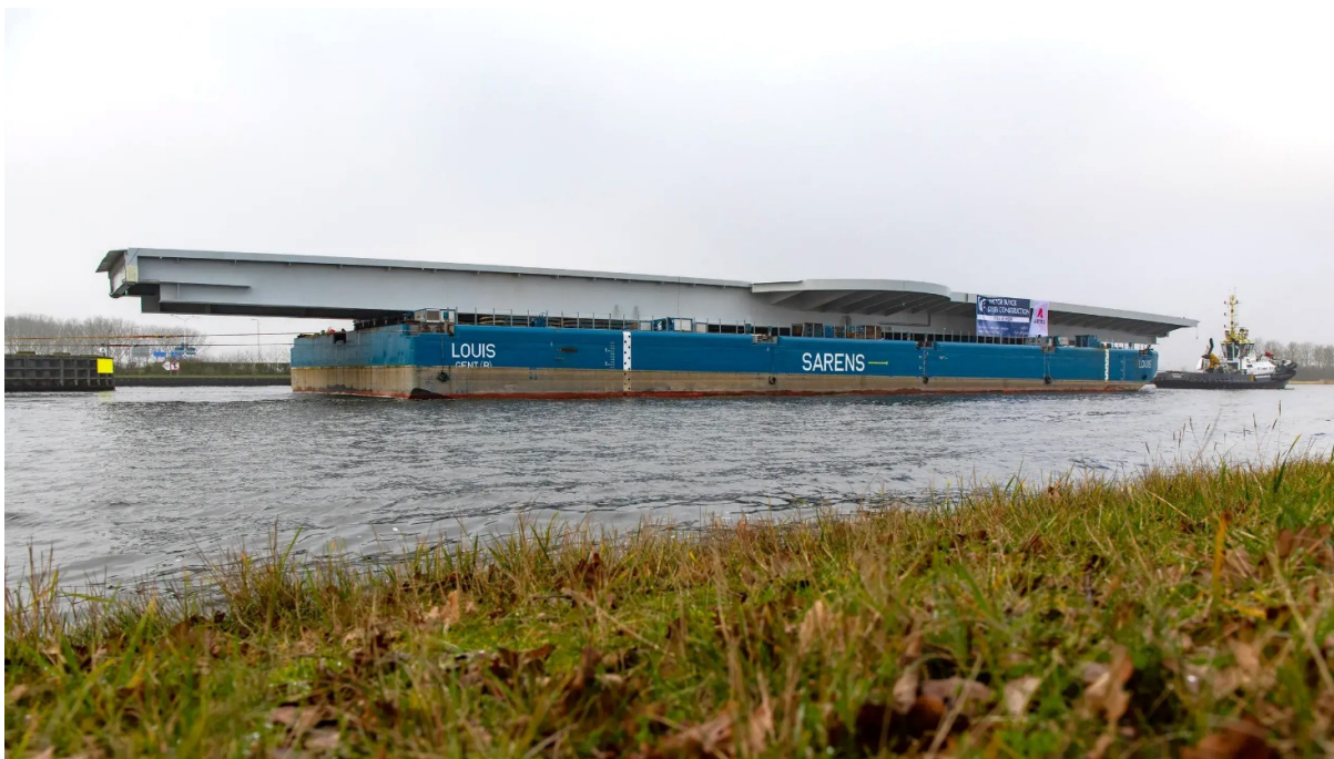
Figure 7: Mobile deck and carousel on Louis 300ft barge after transferring it from Karel and Victor twin barges, starting its sail to the final position at Zeebrugge.
