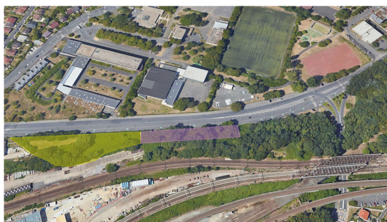
Figure 5: Old bridge demolition area and SPMTs' path
