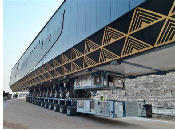
Picture 3: Inclination compensation with SPMT
