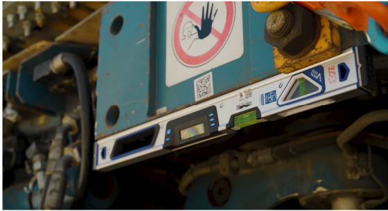
Picture 4: Solar boat live inclination monitoring
