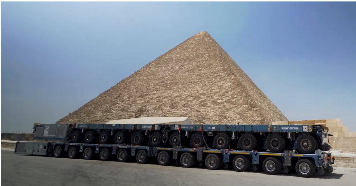
Picture 6: 15 lines of Kamag K24 SPMT's placed on Kamag K25 SPMT's
