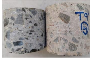
Figure 11. Temperature effects on colour: 100 °C (left), 500 °C (right)
