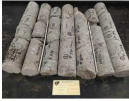
Figure 10. View of some cores extracted from columns
