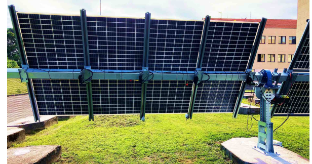
Figure 2. Structural elements of a SAT: torque tube, panels, purlins, pillars and driver.
