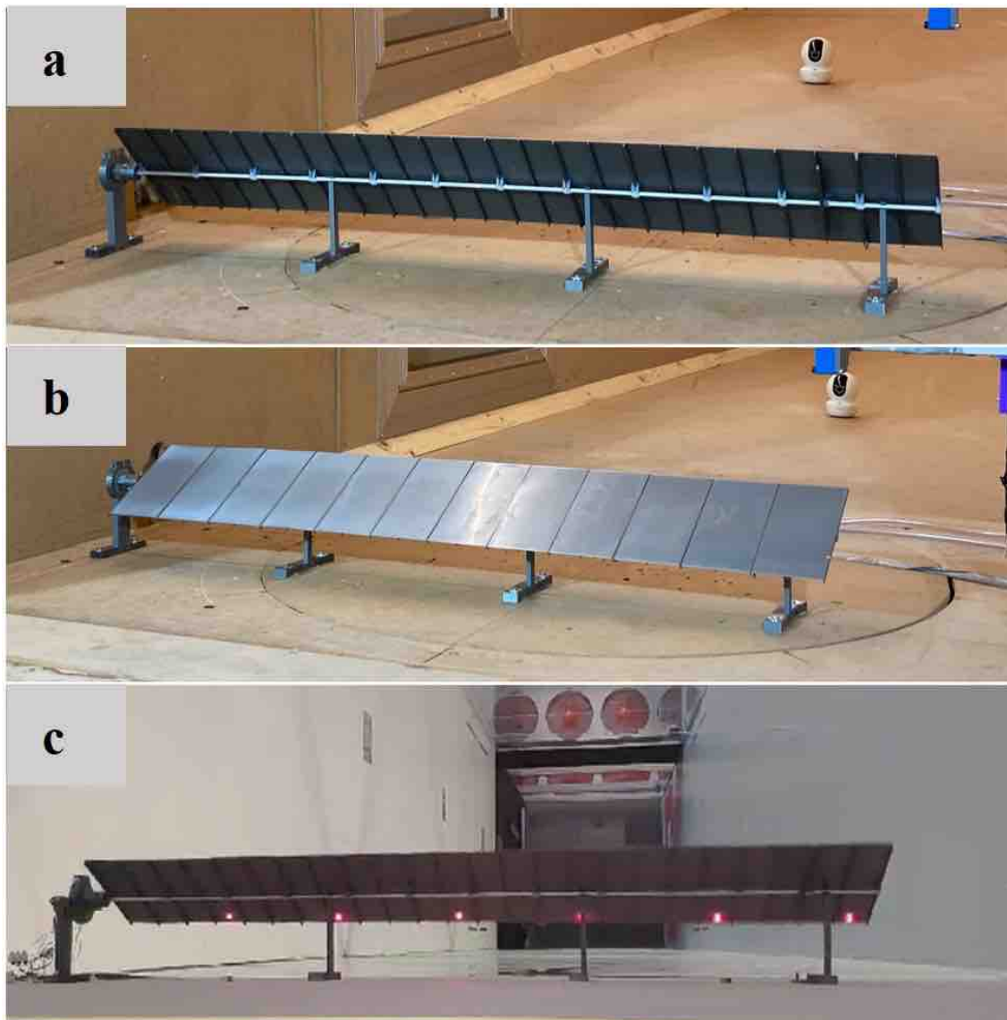
Figure 7. Tracker setup in the test chamber; a-b) University of Oviedo; c) UPM IDR, Madrid.
