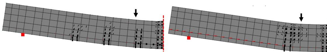
Figure 7. Crack patterns in corroded beam B116 at flexural failure (*left*) and at bond-slip failure (*right*).
