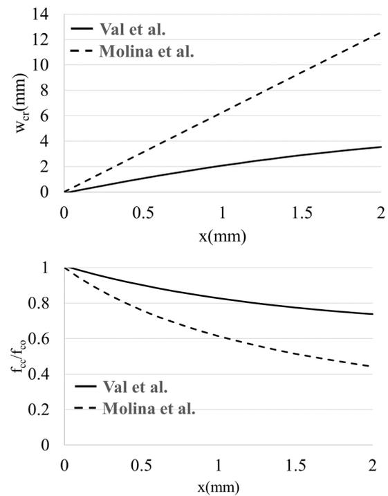
Figure 3. Corrosion-induced crack width as a function of corrosion penetration for Val et al. and Molina et al. models (top) and corrosion-induced compressive strength reduction according to equation (3) (bottom).
