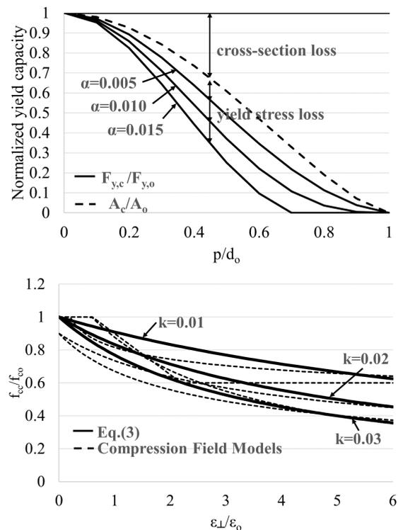
Figure 2. Normalized yield capacity due to pitting corrosion for different values of  $\alpha$  (top), concrete compressive strength reduction due to corrosion cracking and comparison with compression field models (bottom).
