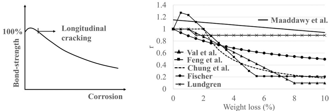
Figure 4. *Left*: Reduction of bond strength between reinforcement and concrete (adapted from [fib (2000)]) as a function of corrosion; *Right*: comparison between used models for bond reduction, with  $r$  being the ratio between maximum bond strengths in corroded and non-corroded stat
