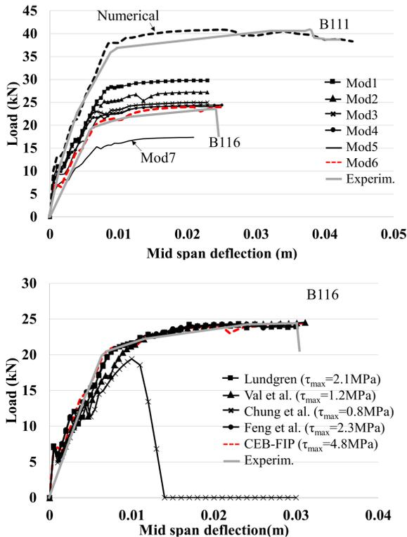
Figure 6 *Top*: Load deflection results for beams B111 (non-corroded reference beam) and B116 (corroded beam); *Bottom*: sensitivity results for beam B116 comparing different models for degradation of bond between reinforcement and concrete under corrosion).
