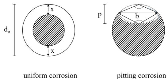
Figure 1. Modelling uniform and pitting corrosion of single reinforcement bar (effective cross-section of the corroded bar equals to the shaded area).
