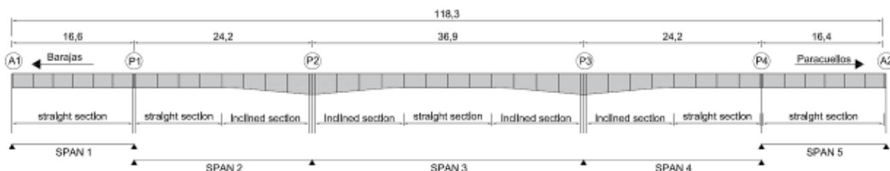
Figure 2: Jarama Bridge Elevation
