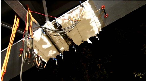
Figure 12: Heating procedure for post-curing.
