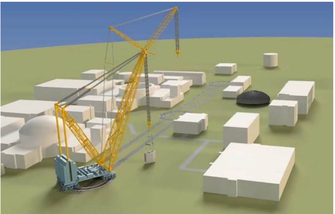
Figure 12: SGC-250 lifting locations at Hinkley site
