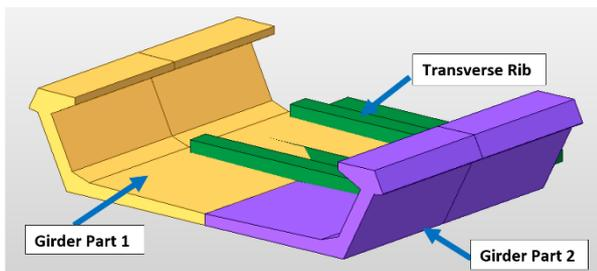
**Figure 9. Section through girder showing half section and transverse ribs**
