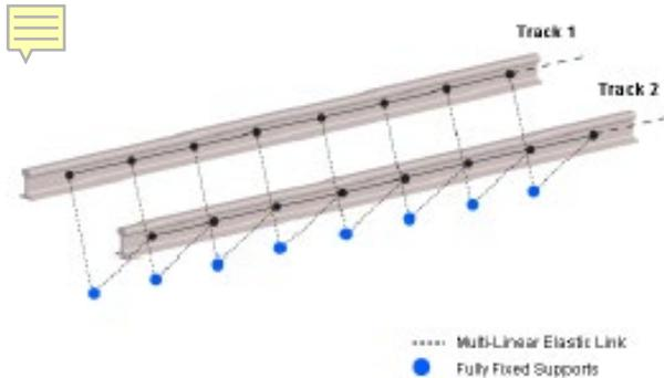
Figure 16. Model of track structure connectivity
