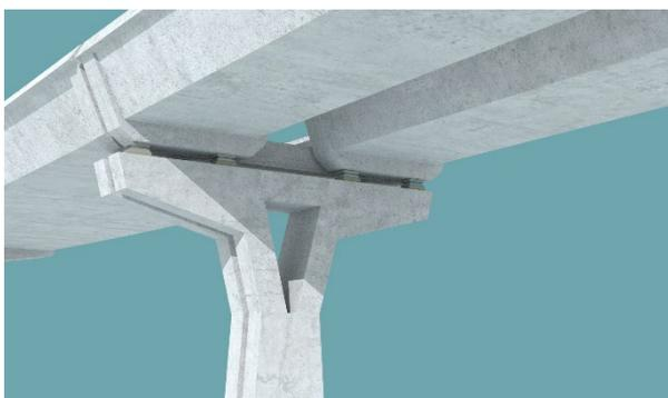
**Figure 3. Concept development of hammer head pier at bifurcating tracks**
