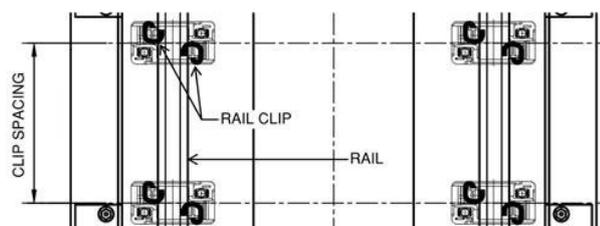
Figure 17. Direct fixation on Elevated Guideways, typical plan view of rail-clip assembly
