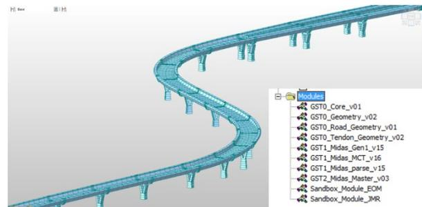
Figure 7. Midas Civil analysis model through VBA
