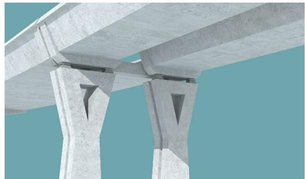
**Figure 4. Concept development of double pier at bifurcating tracks**
