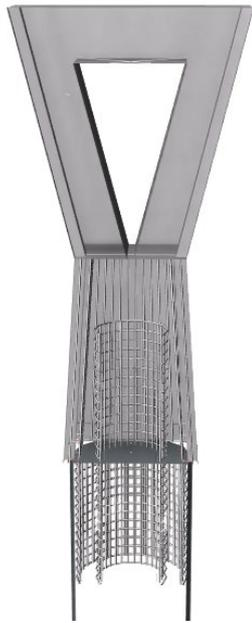
**Figure 5. 2.5m dia. drilled mono shaft to pier connection**
