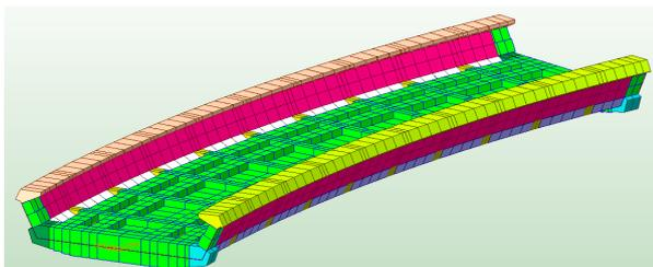
**Figure 10. Transverse analysis model of a typical span**
