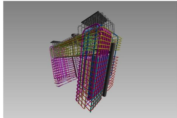
Figure 15. 3D Pier reinforcement model
