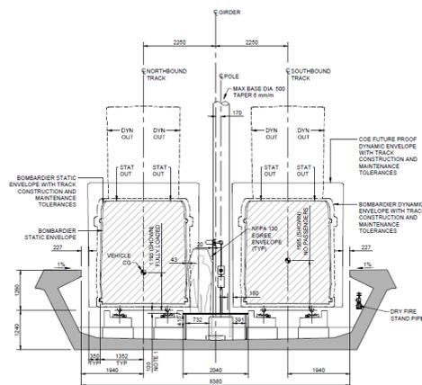
**Figure 6. Guideway functional cross section**
