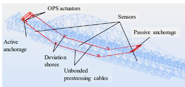
**Figure 5. Main components of the OPS [28].**
