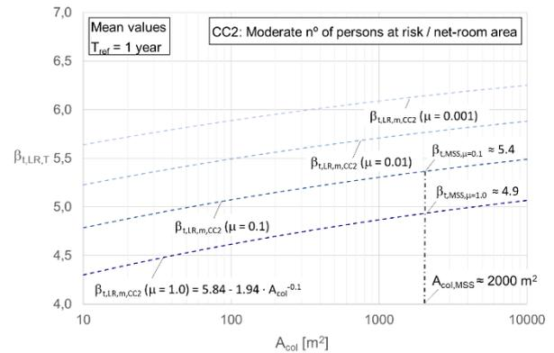
**Figure 1. Target reliability index ( $\beta_{t,LR,T}$ ) for members in temporary structures, belonging to consequence category CC2 [22], versus the area affected by member collapse ( $A_{col}$ ) based on the mean value of implicitly acceptable risks.**
