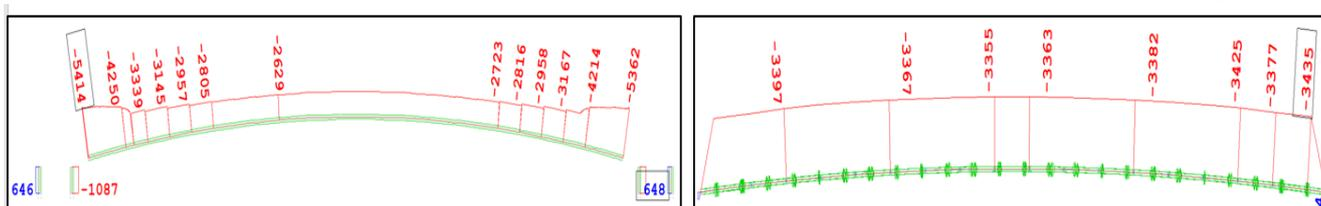
**Figure 8. Main box beam and piles axial forces [kN] under full pedestrian loading (Left)
