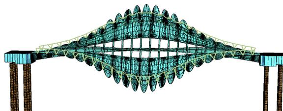
Figure 16. Fourth mode 4.95 Hz (Bending 2)
