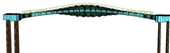
Figure 14. First mode 3.5 Hz (Torsion)
