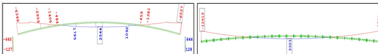
**Figure 7. Main box beam and piles bending forces [kNm] under full pedestrian loading (Left)
