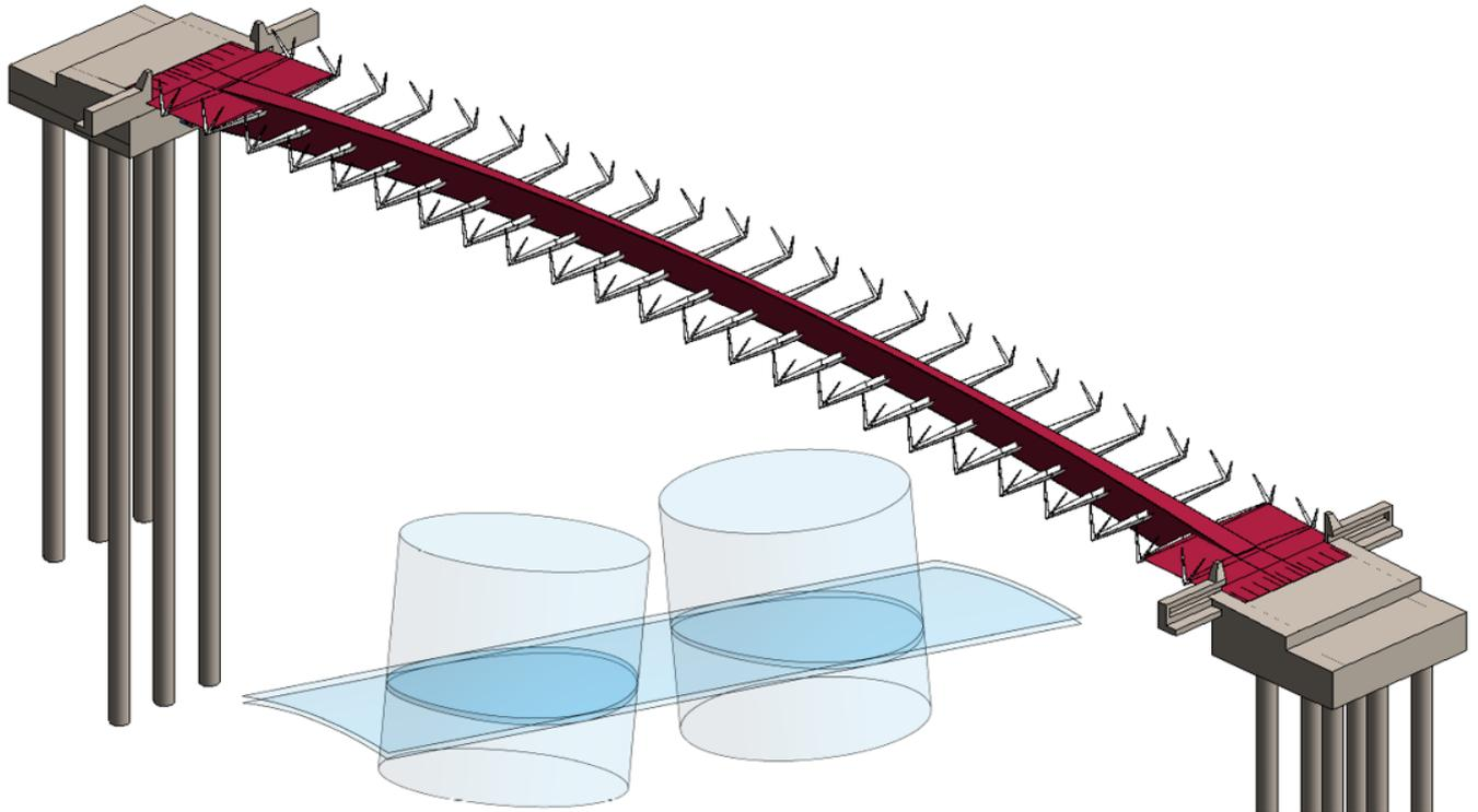
To generate the geometry required for the structural analysis and also the production of the steel drawings from a single source of data, the parametric modelling using Rhino and Grasshopper produced by the architect was transferred to Dynamo for the drawing production and Sofistik for the modelling by developing specific scripts and programming code.
