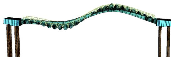
Figure 15. Third mode 4.8 Hz (Bending 2)
