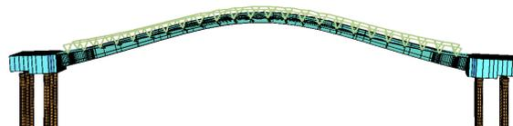
Figure 13. First mode 2.8 Hz (bending)
