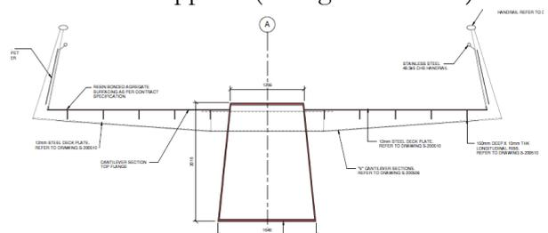
Figure 6. Cross section at supports
