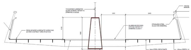
The central box varies in location relative to the pedestrian path but also in width as it follows the large radius cylinders (very close to an inclined plane at  $5^\circ$  inclined to the vertical) this variation in box size increases the transfer of bending moments at supports (see figures 5 and 6).
