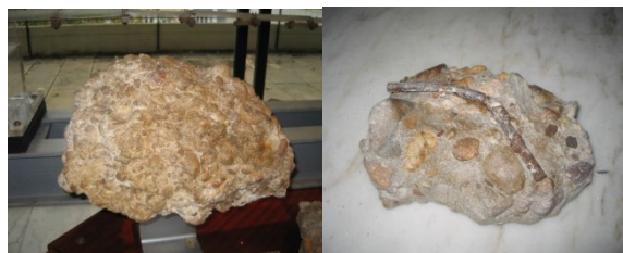
Figure 6: Fragments of roman concrete and of the first reinforced concrete.
