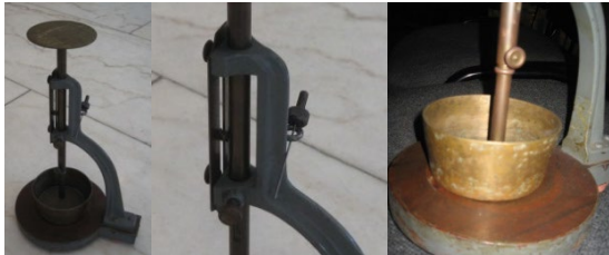
Figure 10: Vicat test tool.
