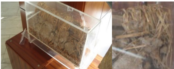
Figure 7: Segment of a earth wall panel.
