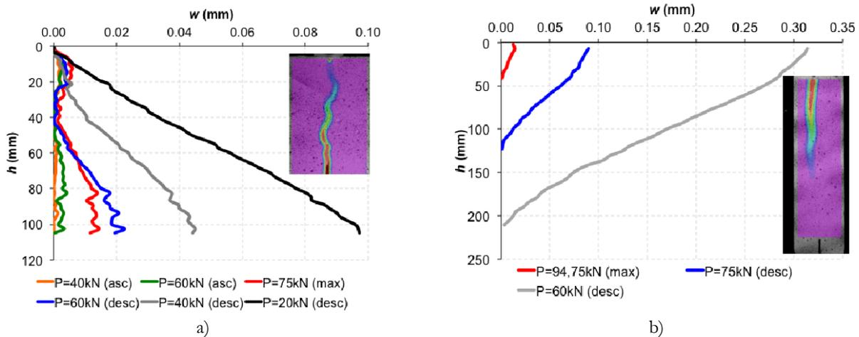
Figure 8. Crack width along the height of the specimen at representative load stages, a) H40/20-150x150x150, b) H40/20-100x100x400
