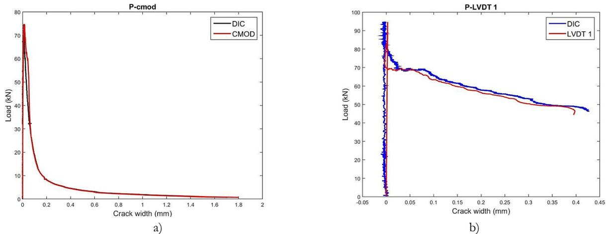
Figure 7. Load vs crack width: comparison between DIC and CMOD results, a) H40/20-150x150x150, b) H40/20-100x100x400
