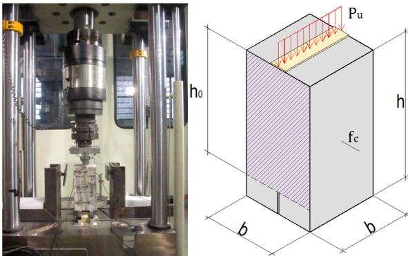
**Figure 2. Test set-up.**
