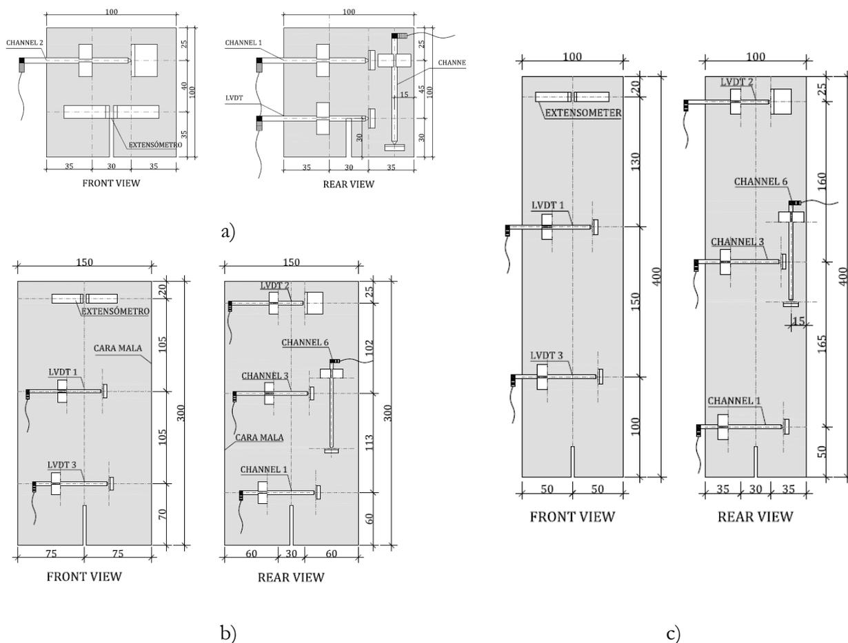
Figure 3. Instrumentation of specimens: a) 100x100x100; b) 150x150x300 mm, c) 100x100x400 mm.
