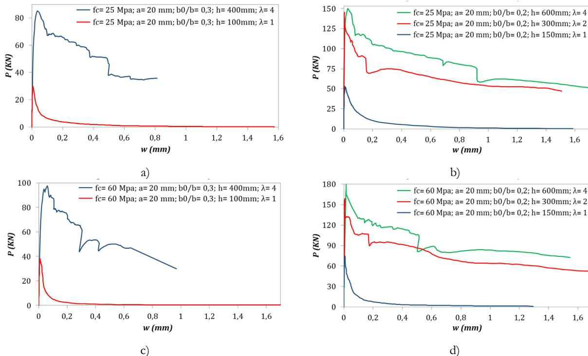
Figure 6. Load vs crack width for different slenderness values
