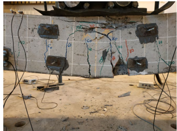
Figura 7. Crack pattern at failure of beam T6a.
