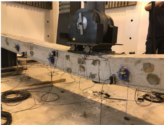
Figura 6. Crack pattern at failure of beam T4a.
