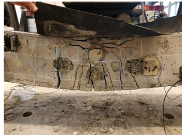
Figure 5. Crack pattern at failure of beam T3a.
